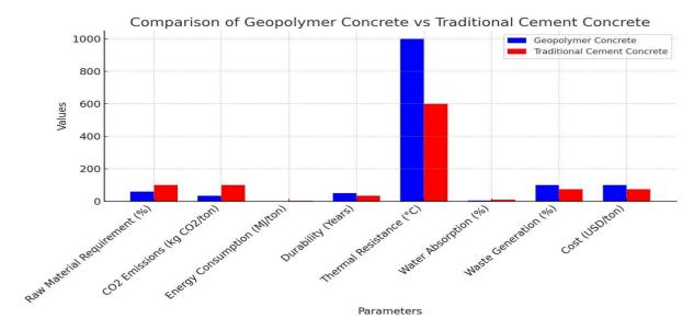
CO2 Emissions Comparison: This bar chart compares the CO2 emissions per ton of material produced by both concrete types.
